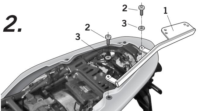
Assemble the kit top support (1) using washers (3) and screws (2).
