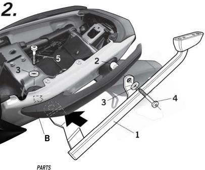
**GB** Assemble the Kit Top support (1) at the same time, assemble the lateral handrails (B) by means the spacers (2), washers (3) and the screws (4) in the front area by means the washers (3) and the screws (5). Assemble the seat (A).
