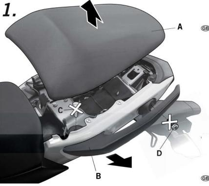
GB Disassemble the seat (A). Disassemble the lateral handrails (B) and remove the screws (C) and (D).
