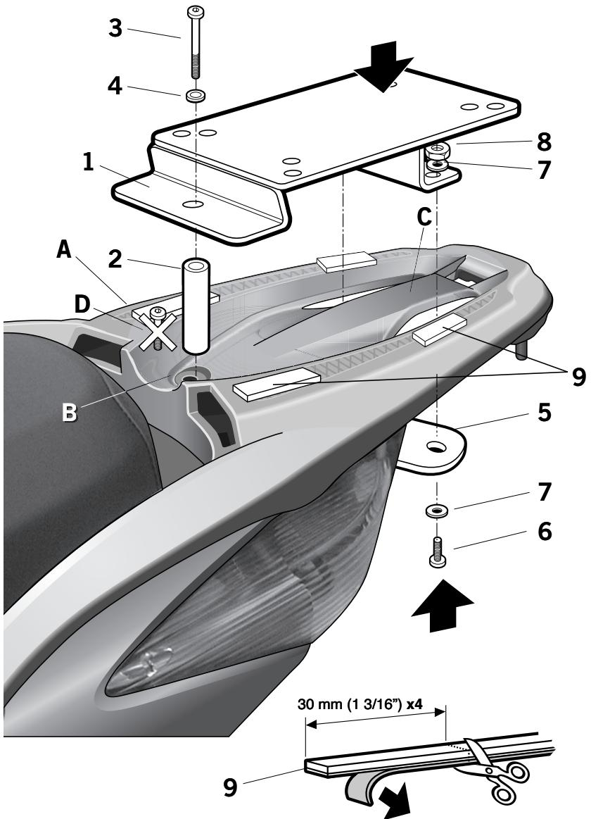
Dismantle and remove the screw (D). Put the adhesive rubber (9) as show in the draw in order to protect the fairing. Assemble the KIT TOP support (1) on the original fold-back seat (A) of the motorcycle and fix it in area (B) using the distance piece (2), the screw (3) and the washer (4). And in area (C) using the flange (5), the screws (6), the washers (7), and the nuts (8).
