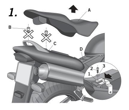
Dismantle seat (A). Unscrew and remove screws (B) from the rear handgrip area (C). Attach pieces (1) on the chassis bracket, area (D) and fix using screws (2) and washers (3). Attach seat (A).
