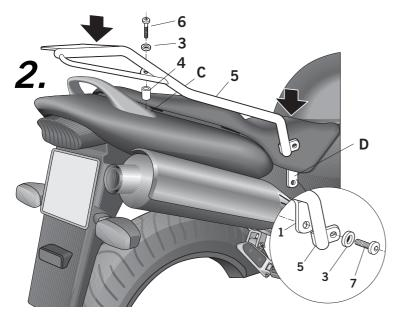
Attach KIT TOP supports (5) in area (C) using spacers (4), screws (6) and washers (3). And in area (D), with pieces (1), using screws (7), and washers (3).
