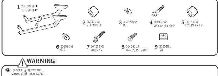
screws until it is ensured that the KIT is correctly attached and aligned.
