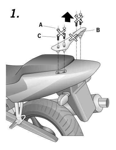
**Proper kit assembly:** do not tighten the screws until ascertaining that the kit is properly positioned and aligned.
