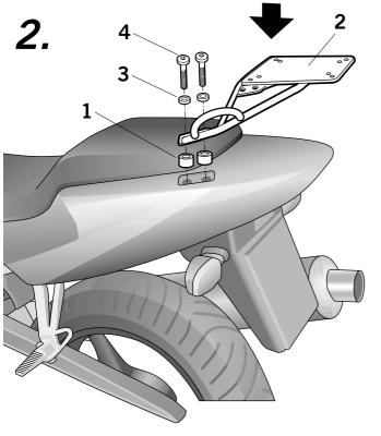
Position the spacers (1). Put the Top Kit base (2) in place using the washers (3) and the screws (4).
