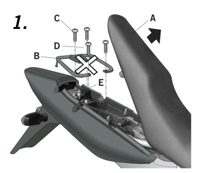
Disassemble the seat (A).
