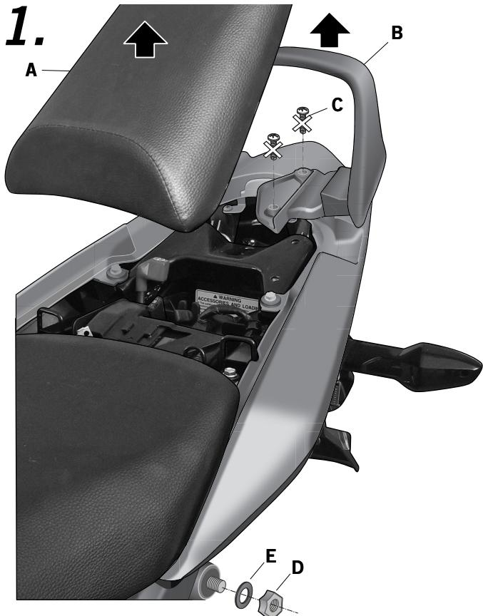
**Advice for correct fitting of the kit:** Ensure that the kit is correctly fitted and aligned before fully tightening the screws.
