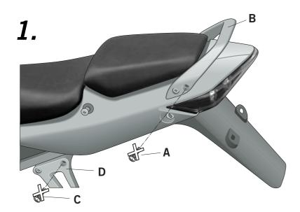
Disassemble and reject the screws (A) of the rear handle (B).
