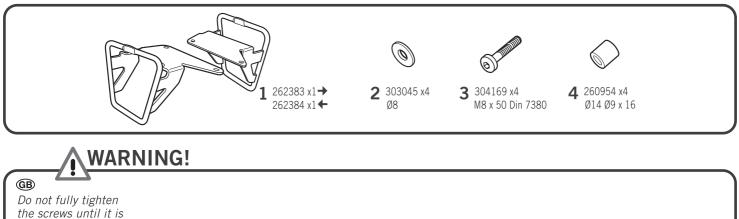
the screws until it is ensured that the KIT is correctly attached and aligned.
