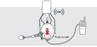
First, connect the two-way radio cable with the headset.
