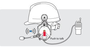
First, connect the two-way radio cable with the headset
