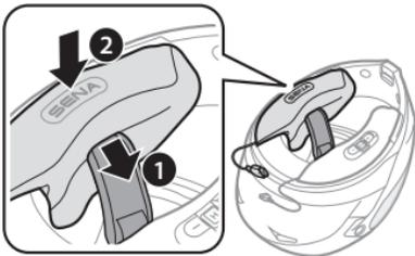
4. Connect the connection cables and store it behind the internal padding of the helmet.
