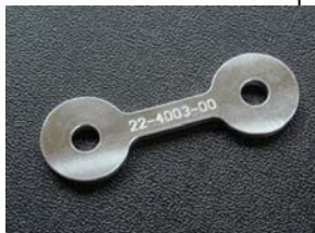
Spacer washer needed on "some" bikes.
