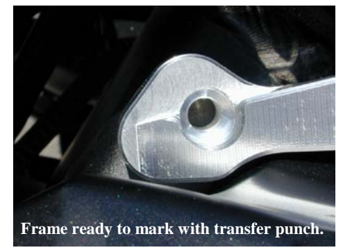
This photo shows the Triple clamp mount (TCM) aligned over the clip-on bolt holes
