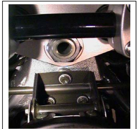
Stock tank bracket before removal
