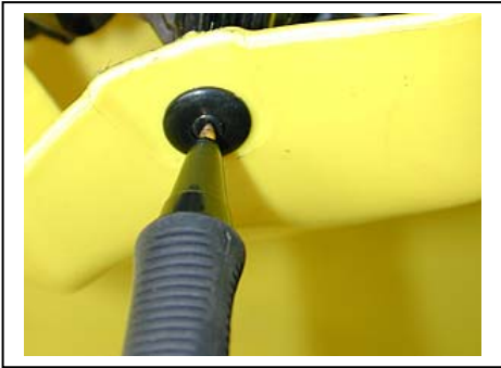
Removing the "push pin retainers"
