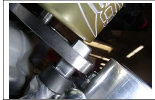
This shows the incorrect tower pin height.
