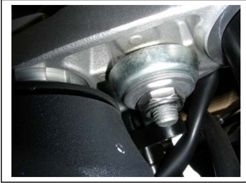
Remove the 17mm nuts under triple clamp
