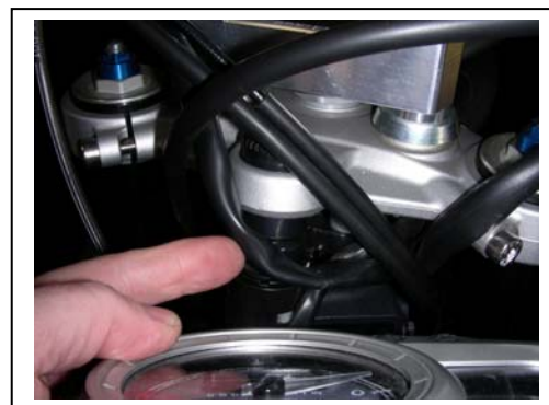
Re-route the wire loom that goes to the right side switches so it's in front of the key cylinder and free to move.
