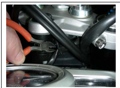
Cut the zip tie holding the wire loom tight to the key cylinder so it can be re-routed as per the photo to the far right
