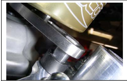
This shows the correct tower pin height
