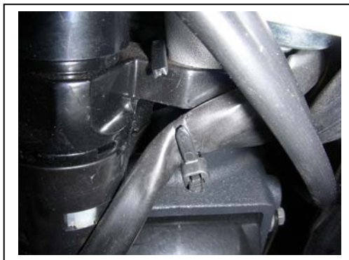
Close up of where to cut the zip tie that holds the wire loom tight. Re-route the wire loom as per the picture to the right.
