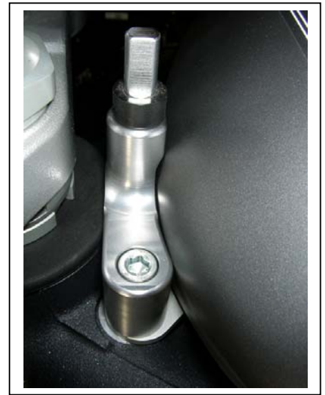
Frame bracket installed into tank mounts Be sure the bracket has clearance to the tank BEFORE you tighten the bolts. In rare cases, it can be filed or shimmed upward using thin washers underneath the frame bracket. Be sure the bolts still engage a minimum of 6mm of thread.
