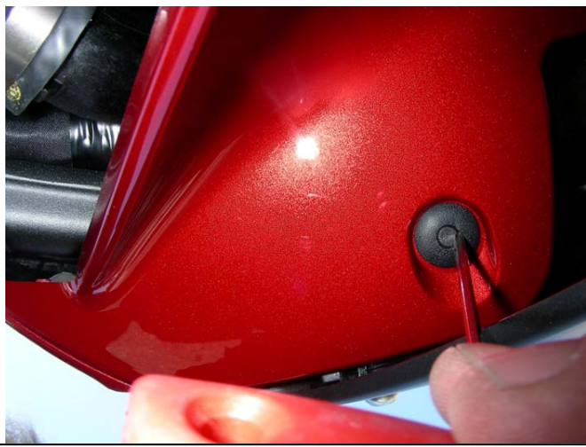
Push on the center of the plastic push pin to release it.
