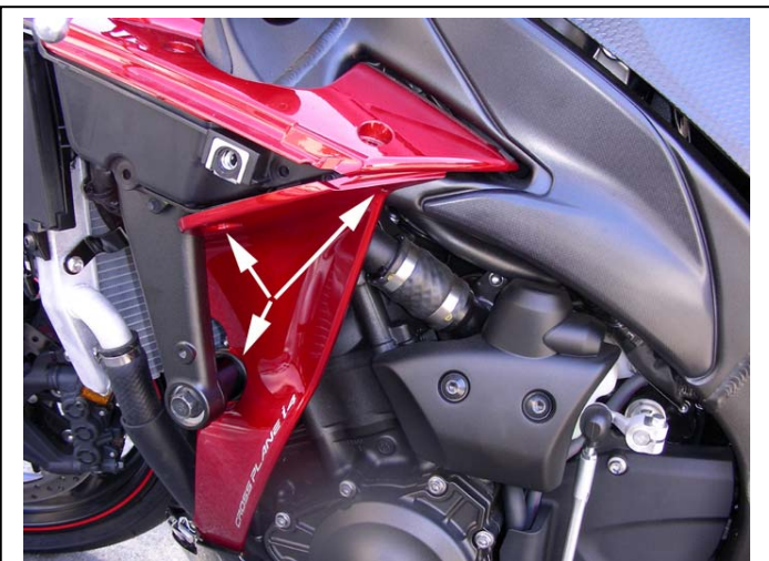
White arrows show the release points for this panel. Rotate this panel back and downward to expose the damper plug
