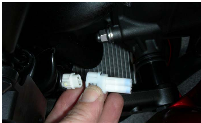
Install the new error code plug we've provided to replace the stock stabilizer switch plug you've undone and removed.
