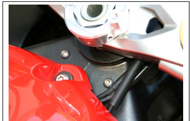
This photo shows the bike with the stabilizer kit removed and the holes plugged. We left them silver in the photo to show you how it looks, although the bolts could be black to blend with the frame.
