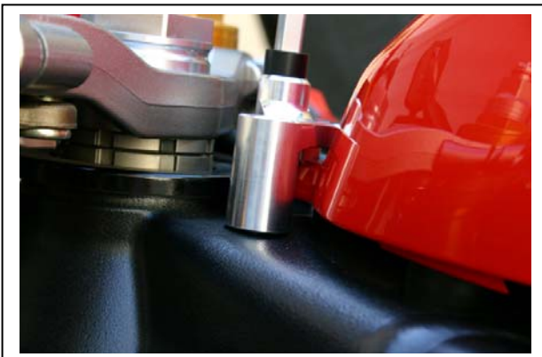
Be sure the triple clamp does not hit the frame bracket at full lock limiting the turning radius.
