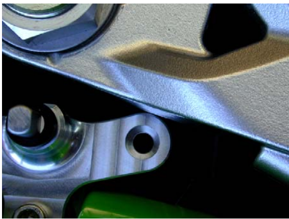
Be sure the triple clamp does not hit the frame bracket at full lock limiting the turning radius.
