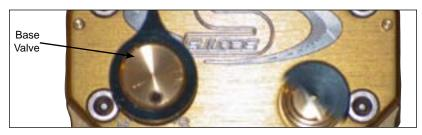
The Base Valve adjusts the amount of resistance you feel as you turn the bars left to right.. As you turn this knob clockwise (to the Right) you will increase the "stiffness" of the stabilizer. Counter clockwise would be less stiff, a softer feeling.
