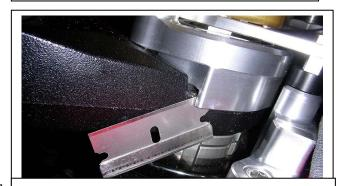
Keeping the TC mount straight while tightening.
