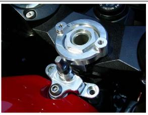
Mounting kit installed, before the stabilizer goes on.
