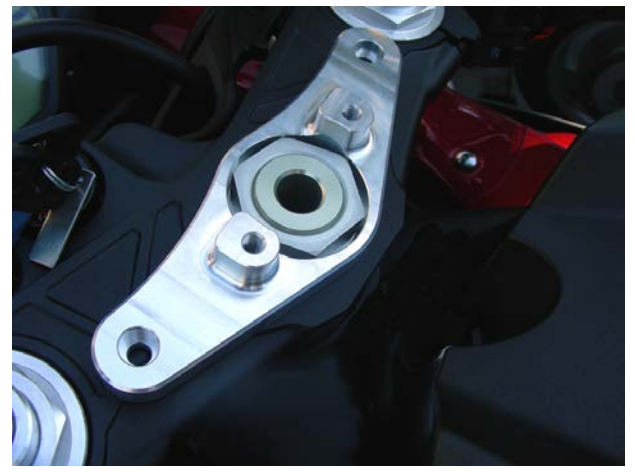
This photo shows the Triple clamp mount (TCM) aligned over the clip-on bolt holes
