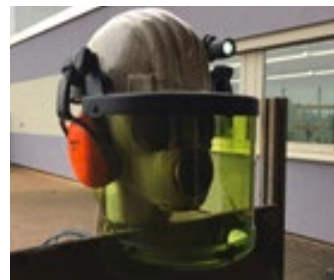
ARCSHIELD before arc flash incident
