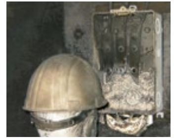
BOP ENERGY 3000 after arc flash incident
