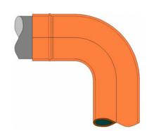
The hose should then push on to the pipe work with some resistance ideally until at least 30mm of hose is past the formed bead.
