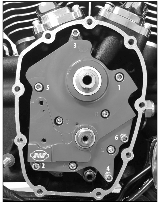
Picture 3a: Cam Plate Screws-Torque According to Step 20
