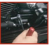
3. Compare the factory shift rod length to the RSD shift rod length. If the length is correct you are ready for installation. If the length needs to be adjusted, loosen the jam nuts using a I/2" wrench and rotate the ball joints in or out to desired length.
