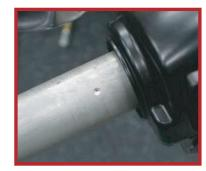
5. Using high strength thread locker and the supplied 5/64" allen key, tighten the two set screws on the grip, make sure the grip is secure. RSD Chrono Grips are supplied with extra badge so pick your favorite style badge to compliment your bike, peel the adhesive backing, and adhere to the end of the grips in a .horizontal position.
