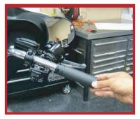
4. With the throttle grip removed, verify the throttle sensor fits correctly on the handle bar then slide the new throttle grip on until the throttle sensor teeth engage. Once installed make sure the flare on the grip fits inside the throttle housing with some room on both sides. If the flange is tight against the throttle housing loosen the master cylinder bolts and reposition to allow the grip to operate smoothly. NOTE: On the RSD Tracker grips make sure the RSD logo is horizontal.
