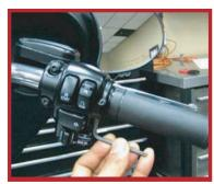
3. Make sure to split the upper and lower switch housing enough to clear the groove on the throttle grip then slide off the throttle grip.
