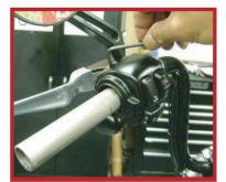
3. Slide on the new RSD clutch grip until the grip stops against the switch housing. Using a I/8" transfer punch and hammer, mark the set screw locations through the threaded holes in the grip. NOTE: On the RSD Tracker grips make sure the RSD logo is horizontal.
