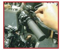
3. Loosen up the throttle and idle cables using two 3/8" wrenches. Make sure to split the upper and lower switch housing enough to clear the groove on the throttle grip then slide off the throttle grip.
