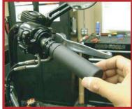
4. Slide the RSD throttle grip onto the handle bar and insert the throttle and idle able ends. Position the upper and lower switch housing on the handle bar. Tighten the 2 Torx T25 screws to factory torque specs. MAKE SURE THE THROTTLE OPERATES SMOOTHLY LOCK TO LOCK. If operation is not smooth loosen the master cylinder and throttle housing and reposition to allow for smooth function.
