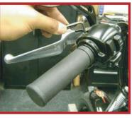
2. Use a long flat blade screw driver to break loose the adhesive between the grip and the handle bar, or cut the grip off carefully. Install the upper and lower switch housing back onto the handle bar and tighten the T25 torx screws to factory specs.
