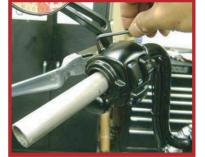
3. Slide on the new RSD clutch grip until the grip stops against the switch housing. Using a I/8" transfer punch and hammer, mark the set screw locations through the threaded holes in the grip. NOTE: On the RSD Tracker grips make sure the RSD logo is horizontal.
