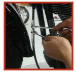
Using a snap ring pliers remove the retaining ring from the pivot pin located on the underside of the clutch pivot housing. Save the retaining ring, it will be reused.
