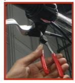
4. Remove the pivot pin, stock clutch lever, and the plastic clutch cable pin. Save these parts, they will be reused.
