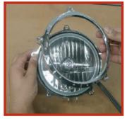
6. Install the supplied I/4" socket head screws (3) using blue thread locker and torque to 8 ft-lbs.
