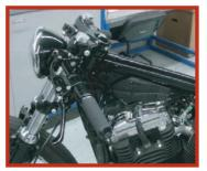
3. With the tank removed, locate the headlight wiring harness connector and disconnect.
