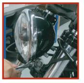
Remove the stock bezel trim using a phillips screwdriver. Keep the headlight assembly in tact since the RSD bezel can installed now.
