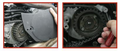
3. Use high strength thread locker on the supplied I/4" socket head bolts and install the RSD pulley cover with the supplied spacers. Torque bolts to 90-120 in-lbs.
