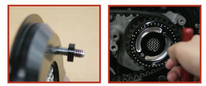
4. Reinstall any components that were removed. Install the RSD Tracker front belt guard 0217-2006 (Sold separately) to complete the tracker look.
