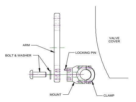
Notice that if you hold the mount and clamp together there is a gap only on one side. This gap should be at the bottom of the engine guards.
