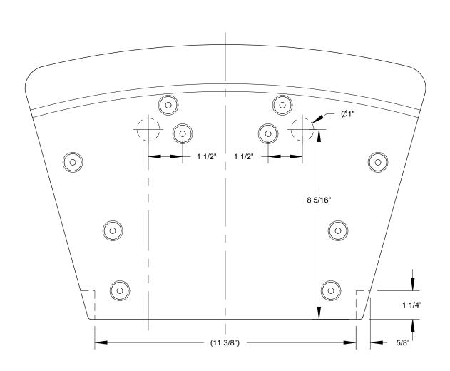
Cut rear corners 5/8" x 1 1/4", and drill or cut the two  $\not O$ 1" holes as shown
