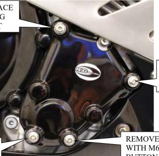
REMOVE AND REPLACE WITH M6x35mm LONG BUTTON HEAD BOLT
