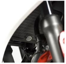
In This Kit There Should Be 1x Radiator Guard (RAD0104BK) 2 x Cable/Zip Tie 2x 100mm Lengths of self adhesive Foam
