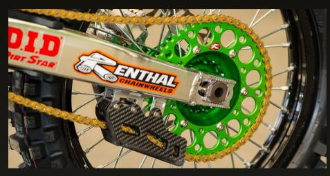
Renthal Ultralight<sup>™</sup> rear chainwheels are manufactured to extremely tight tolerences from a special material developed to withstand the rigours of supercross, motocross and enduro racing.
