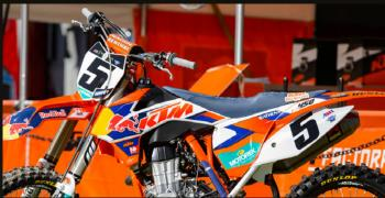
Renthal<sup>®</sup> Fatbar<sup>®</sup> are the market <u>leading unbraced handlebar</u>. Featuring a tapered wall profile enables the clamping diameter(1-1/8" | 28.6mm) to be larger than the control ends (7/8" | 22.2mm).
