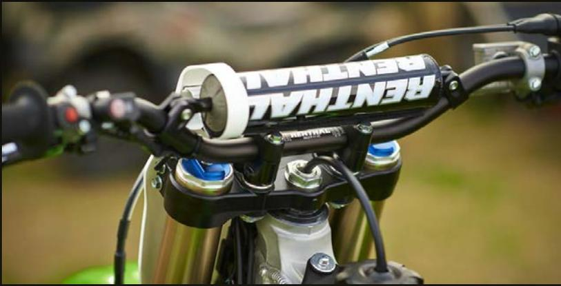
Renthal employs extremely close tolerances and an exclusive alloy, specifically developed for the manufacture of handlebars with specific properties that help limit vibration (a common cause of rider fatigue).
