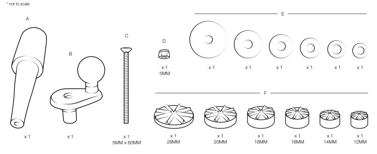
Measure inside diameter of fork stem to determine which side of the (A) expansion plug your install requires.
