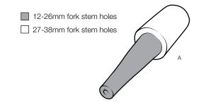
Gently insert the side of the (A) expansion plug that was determined in Step 1 into the stem hole and mark approximately 1/8" above the opening.
