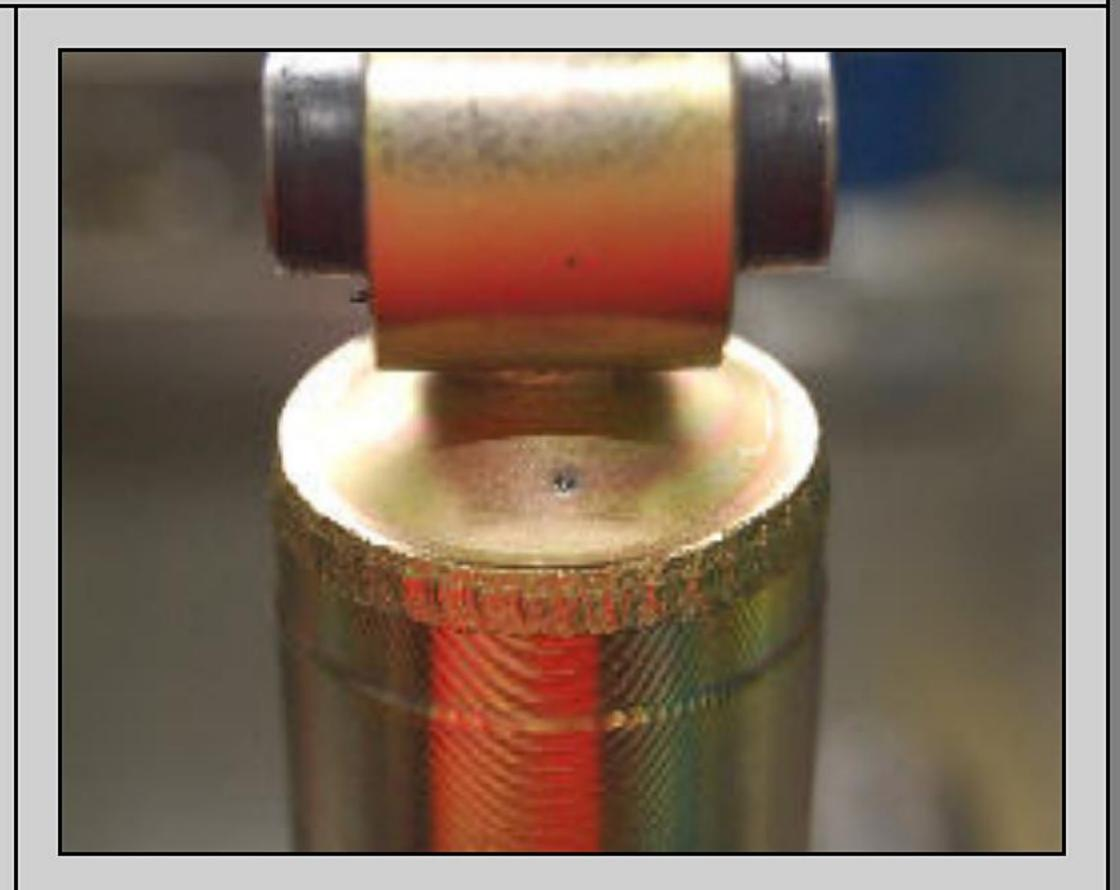
**Note**: In some shocks the reservoir piston or bladder cannot be removed even after the shock is disassembled. In this case the metal chips must be thoroughly removed. Dab a small amount of grease on the end of the drill bit to help catch metal filings.
