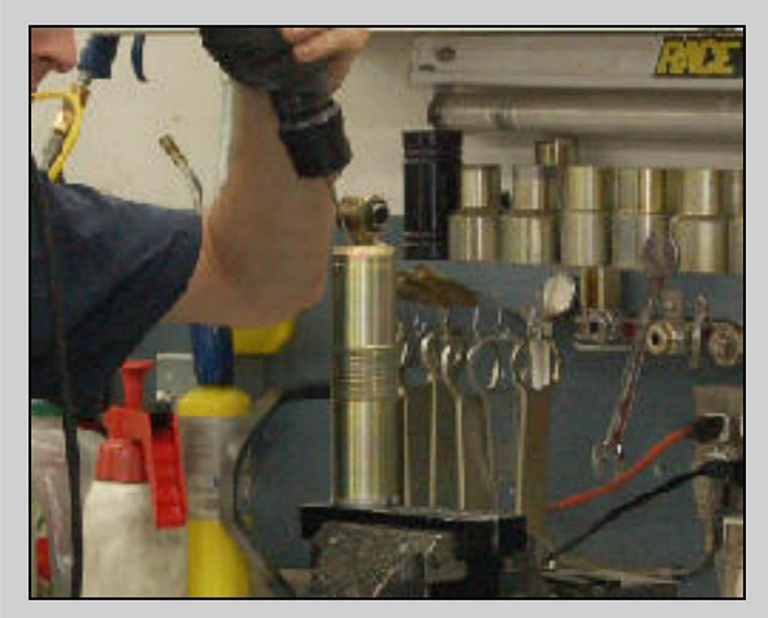
Step 4 - Make a flat where the bolt head must seal by milling or carefully filing.
