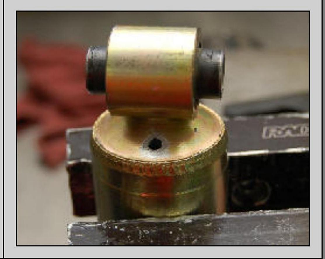
Step 5 - Tap the hole to M5 x 0.8mm
