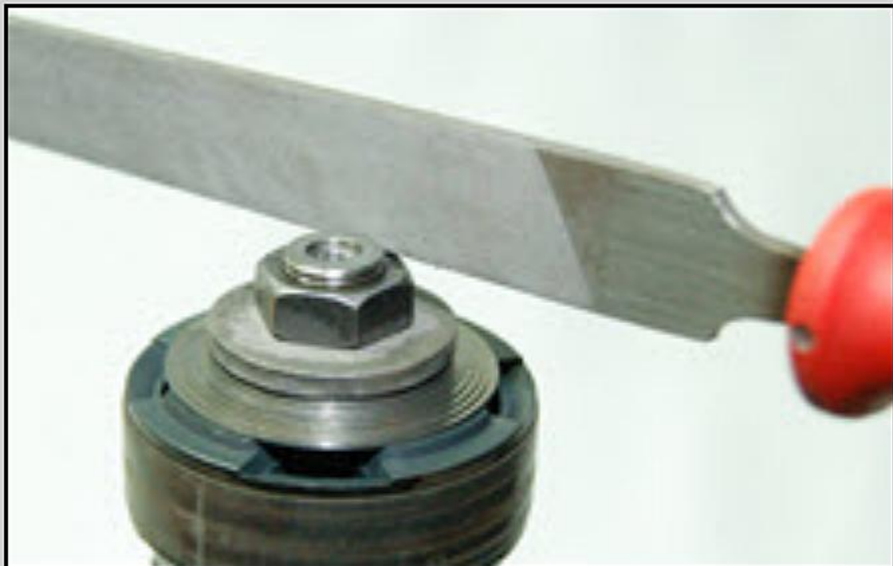
Removing the peening with a file.
