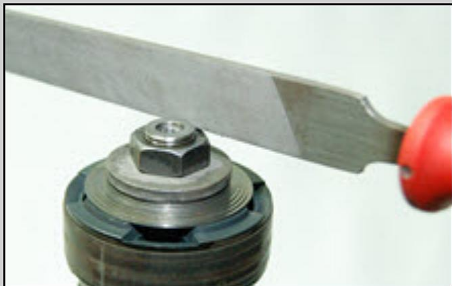
Removing the peening with a file.
