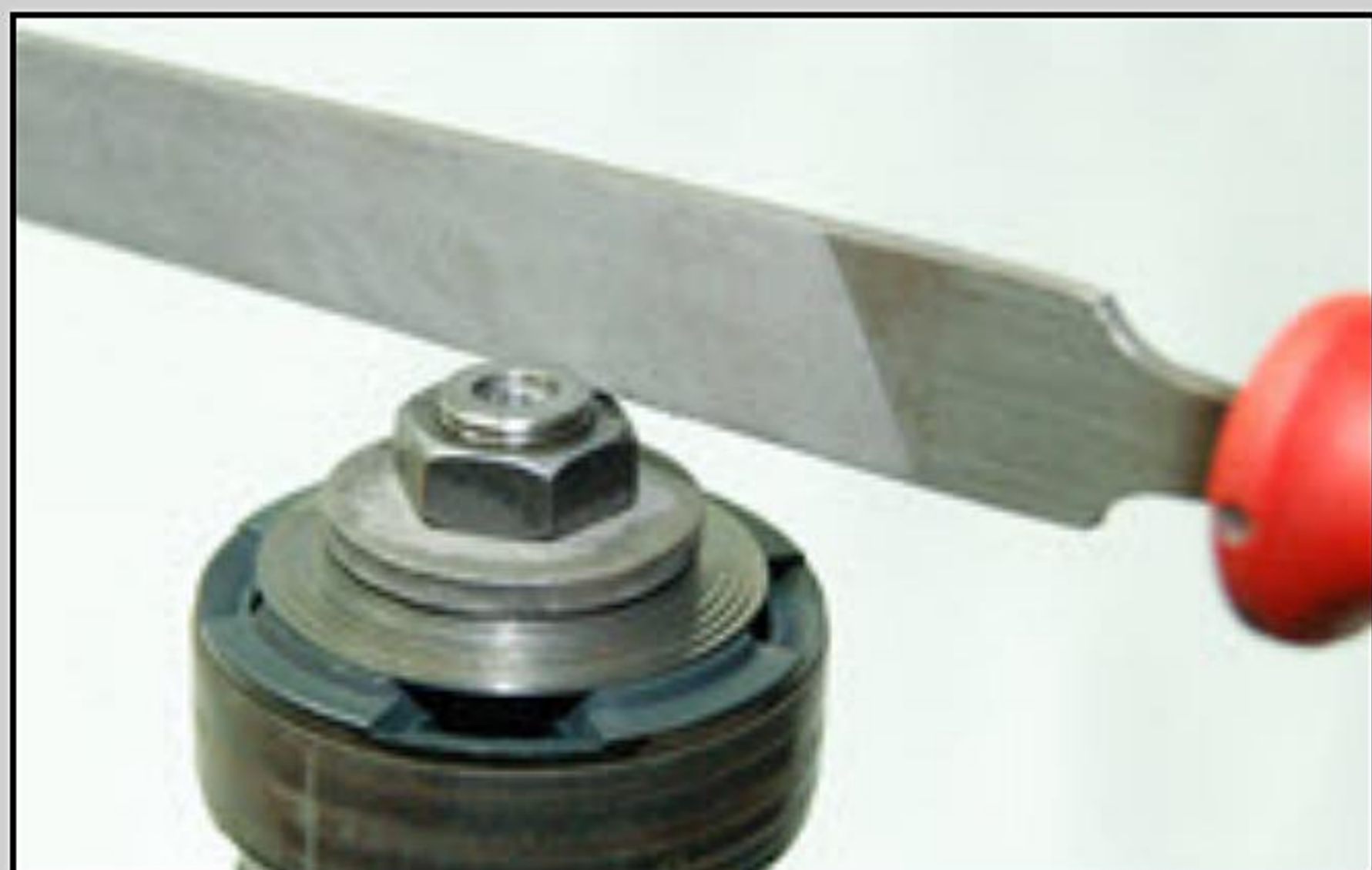
Removing the peening with a file.
