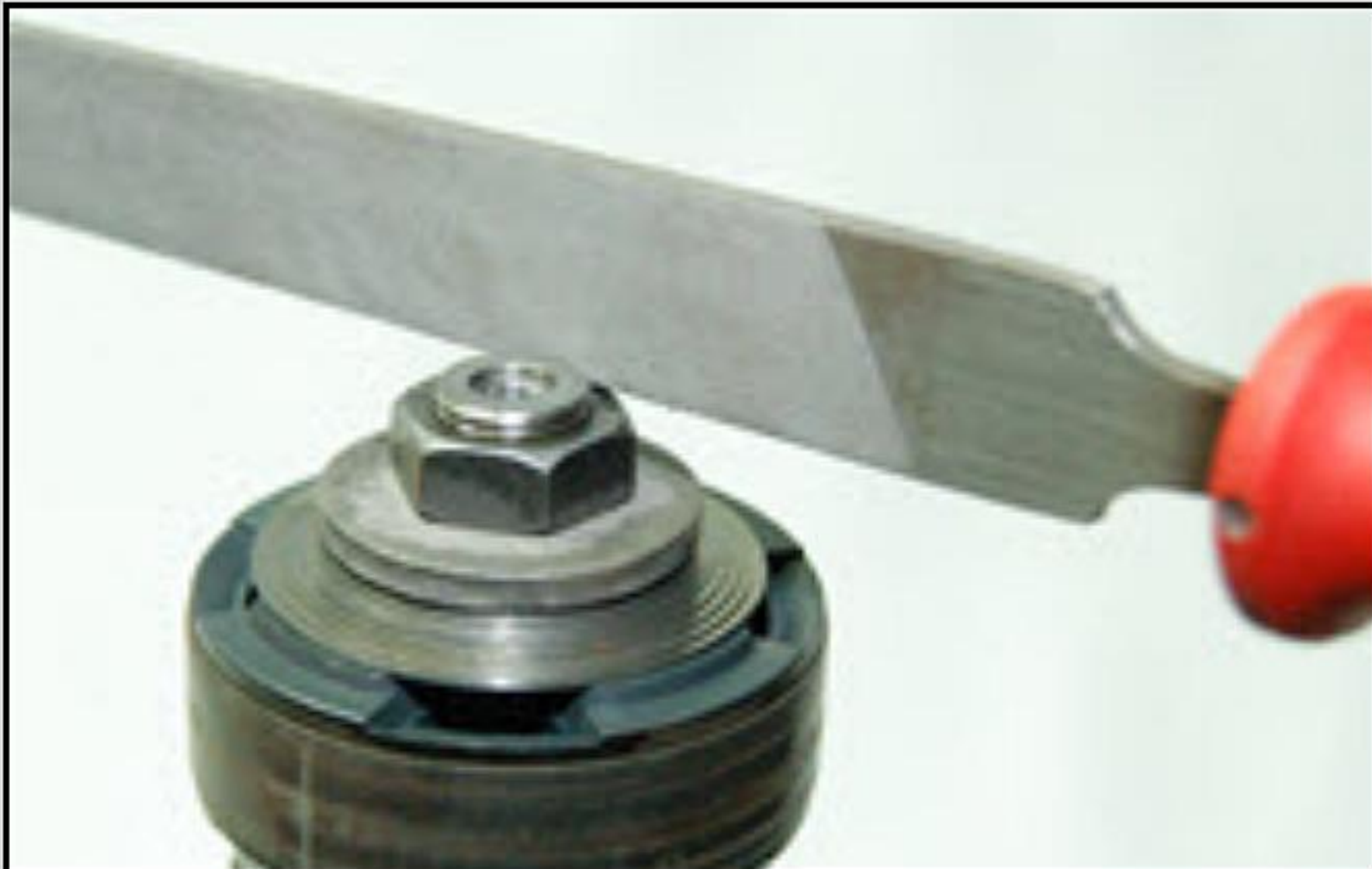
Removing the peening with a file.
