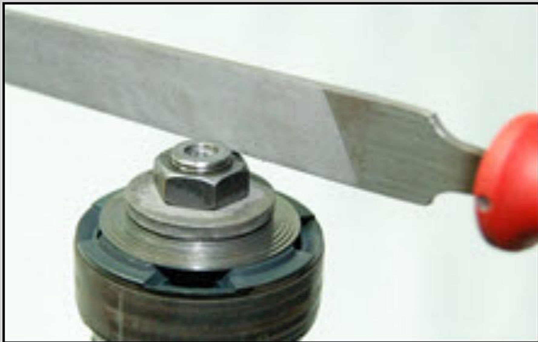
Removing the peening with a file.
