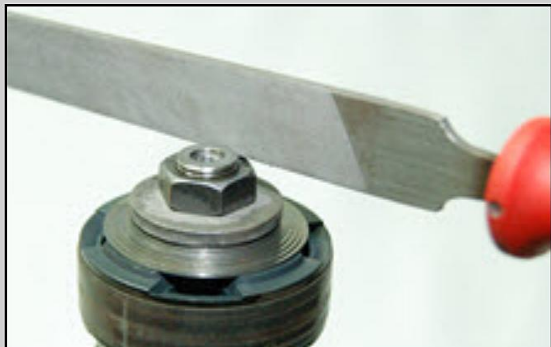
Removing the peening with a file.
