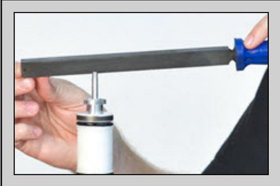
VP3- Slightly chamfer the end of the thread with a fine file. Do not be too aggressive as on some models there is not much thread.
