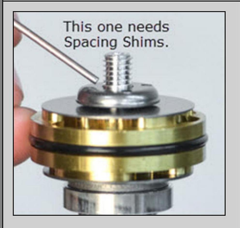
Incorrect stack height is shown in this photo (this stack is too short).
