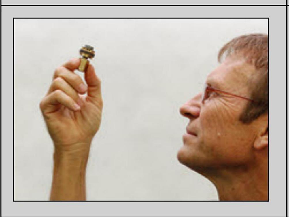
VR16- Check your work. Hold the valve assembly up to the light and look for proper assembly. If there are any problems, disassemble the stack and look for burrs to surface and/or dirt in the valving. Reassemble and check again.
