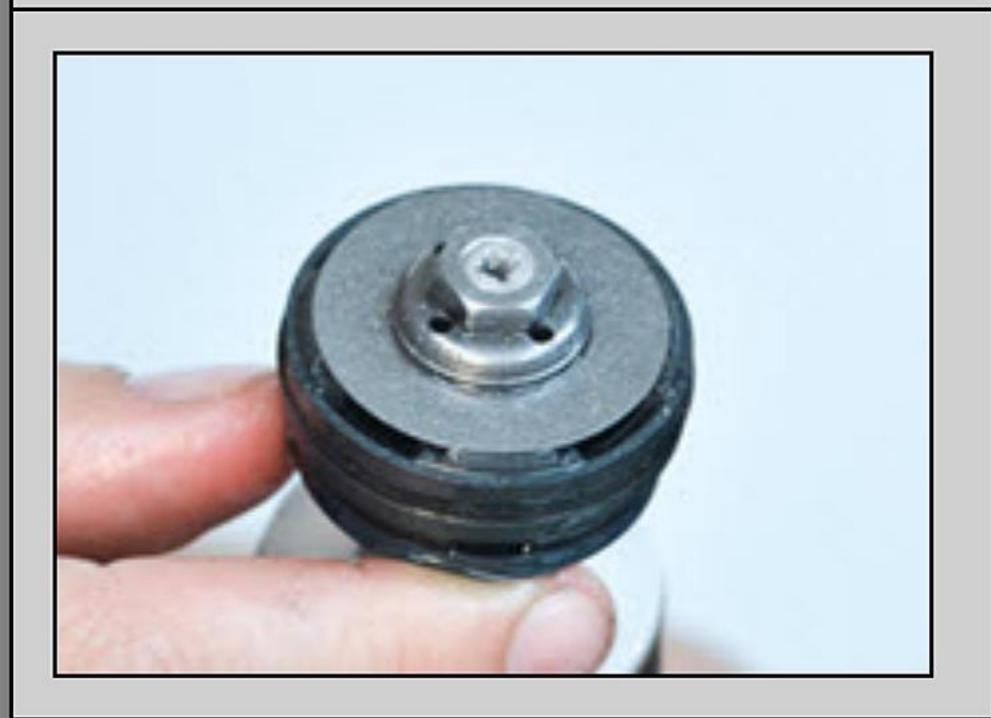
VP2- The shaft should be ground to the nut's surface. Once this is done, remove the nut and Valving Stack.
