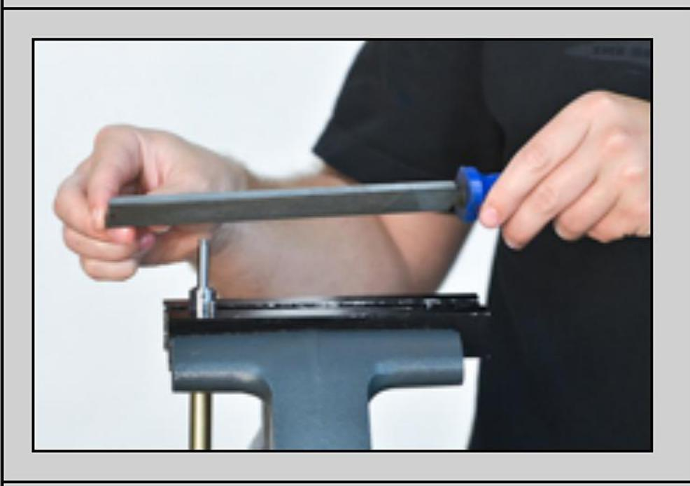
VR4- Chamfer the rebound valving shaft lightly. Use a wire wheel on the shaft end to smooth it.
