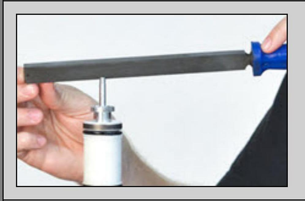
VP3- On peened type holders, slightly chamfer the end of the thread with a fine file. Do not be too aggressive as on some models there is not much thread.
