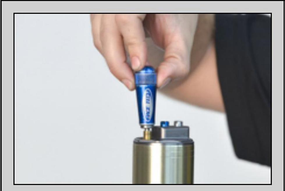
FD3- Using the Race Tech Tool, remove the valve core to release pressure.
