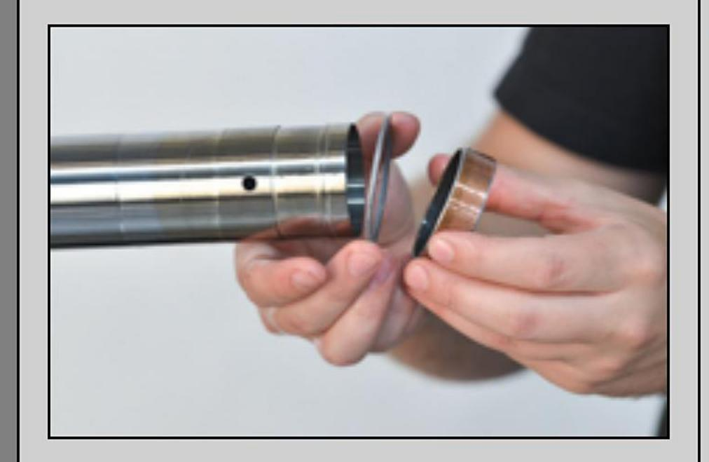
FD22- Remove the bushings and the seal washer.
