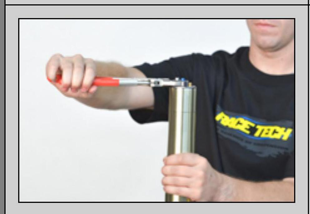
FD4- Remove the fork cap using flat pliers or wrench.
