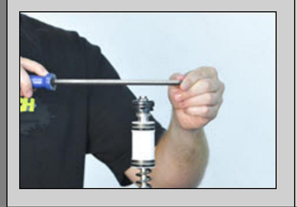
VP1- Most Japanese forks like KYB and Showa have peening on the end of the shaft for nut retention insurance.
