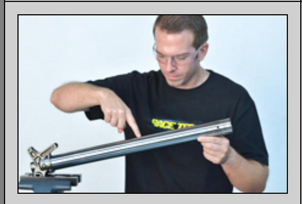
FD25- Inspect the fork tube for pits, dings, and straightness.
