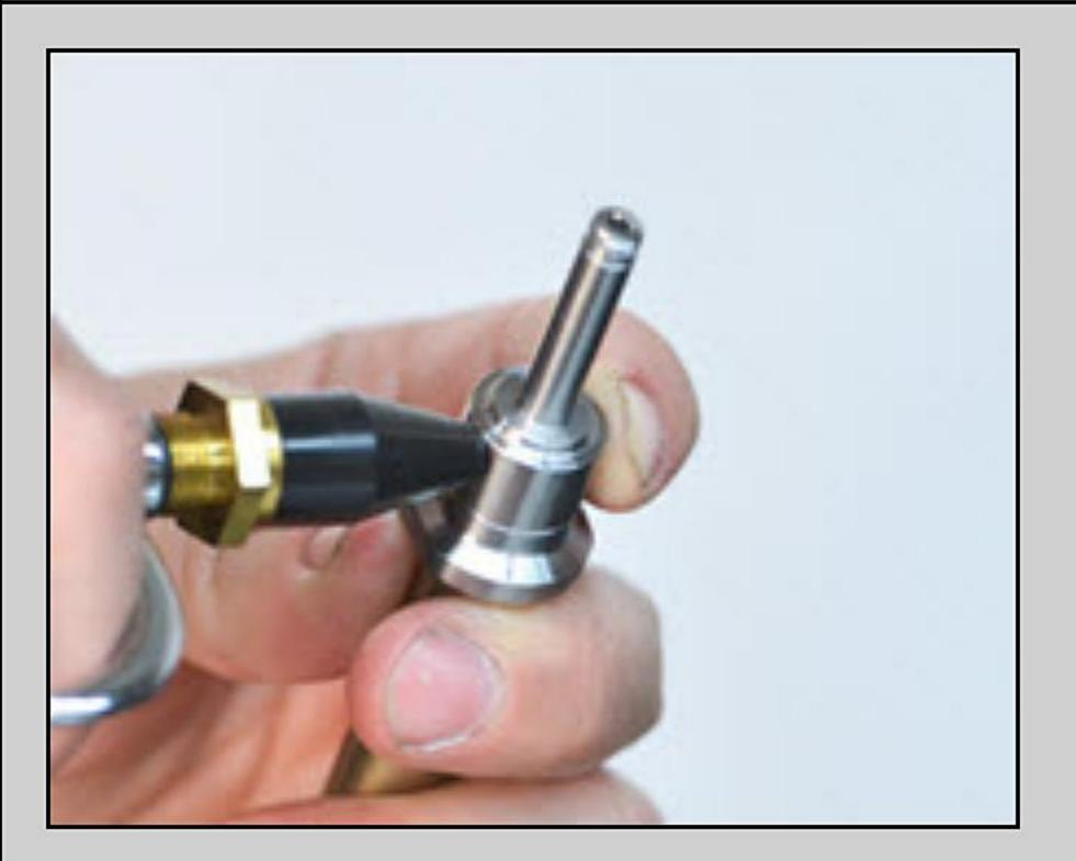
VR5- Blow air through one of the side holes while covering up the other side hole. This allows any fillings that may be in the shaft to be removed through the top hole.
