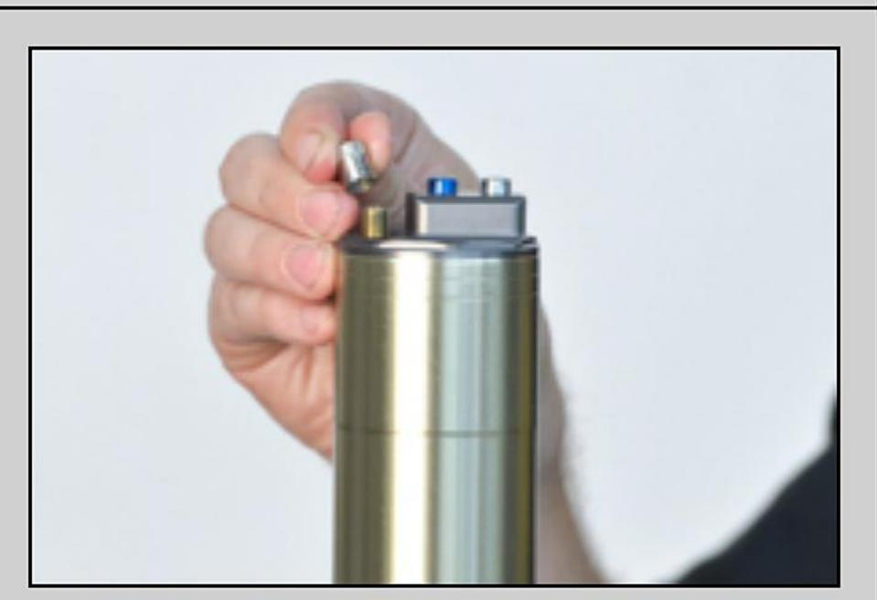
FA12- Install the valve cap.
