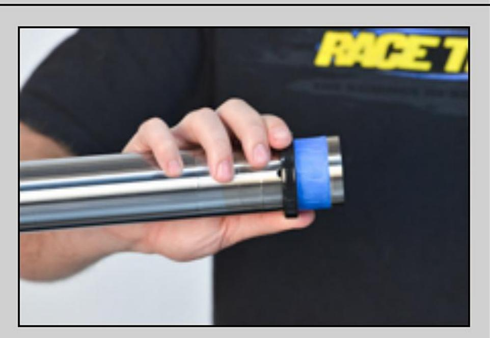
FD23- If you're not replacing seals, use blue painters tape or electrical tape to cover the sharp edge of the bushing groove during removal.
