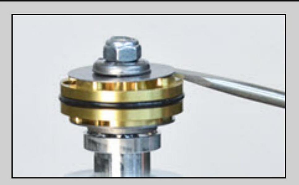
VP13- Check to make sure the check valve is free before the nut is tightened.
