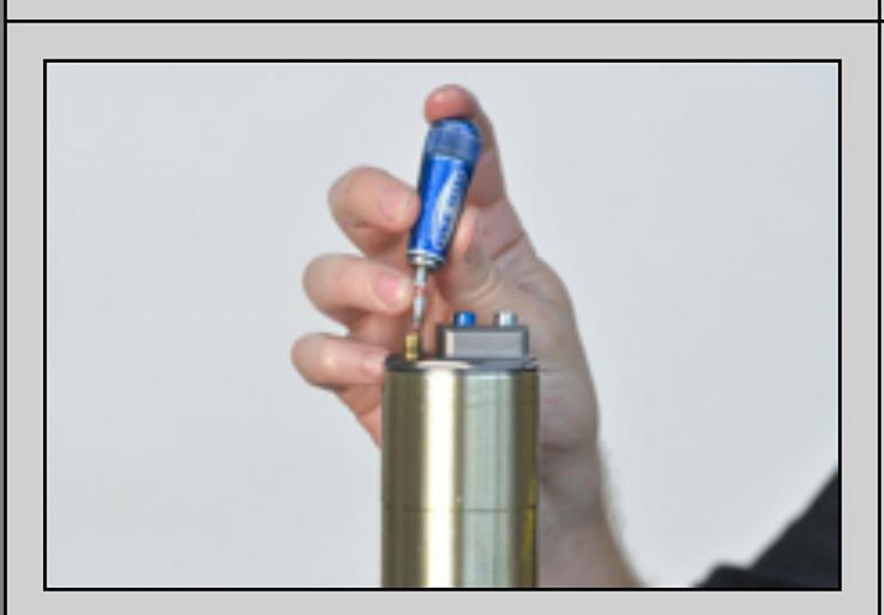
FA10- Install the valve core.
