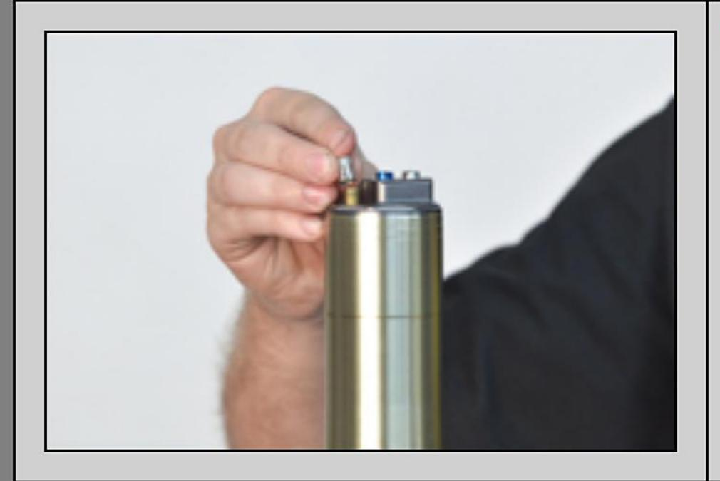
FD2- Remove the valve stem cap.
