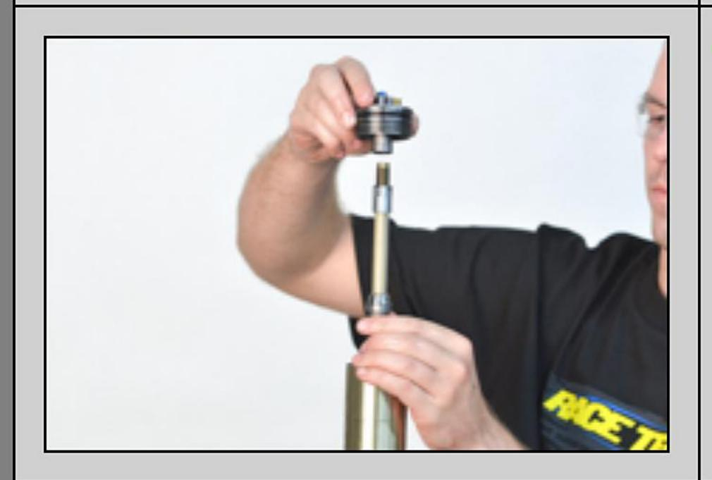
FA7- Install the cap onto the rebound rod.
