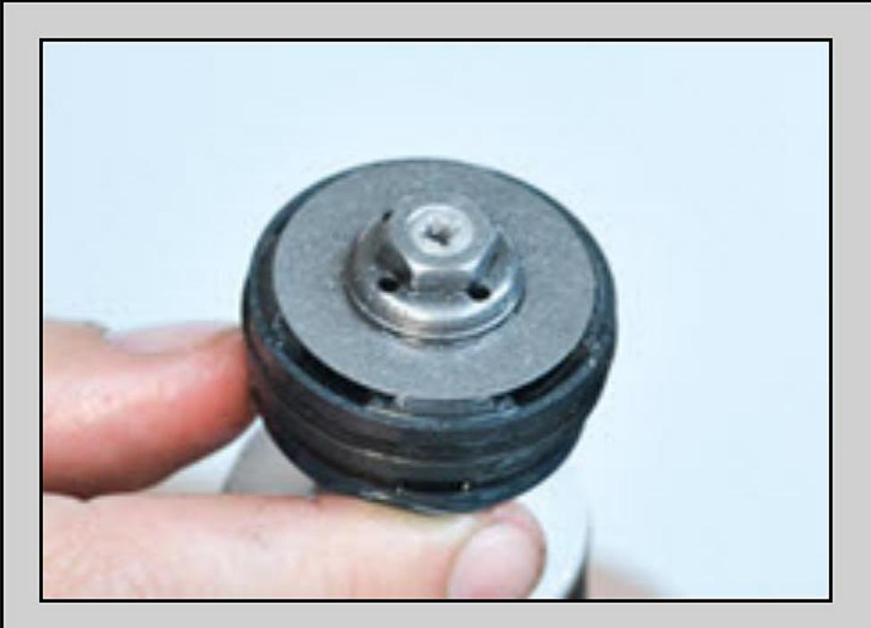
VP2- The shaft should be ground to the nut's surface. Once this is done, remove the nut and Valving Stack.
