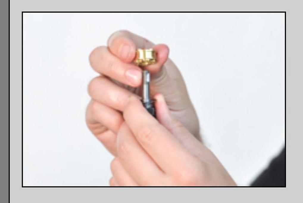
VR9- Install the Rebound Gold Valve WITH THE RECESS IN THE GOLD VALVE FACING DOWN TOWARDS THE MID-VALVE.
