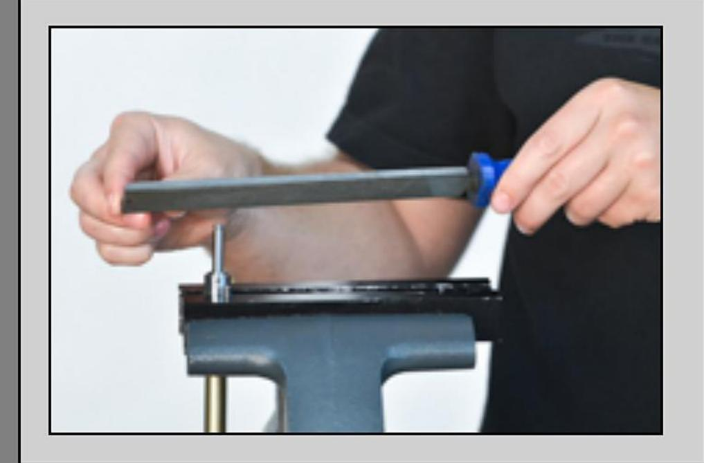
VR4- Chamfer the rebound valving shaft lightly. Use a wire wheel on the shaft end to smooth it.
