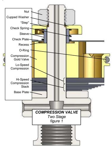
it does, the nut will not tighten down on the valving. This will cause incorrect operation or the nut will come off. This is a critical part of the installation. To get the proper total valve stack thickness you may need to place some of the original shims on the shaft just after the base plate. NOTE: Any shims added must be larger in diameter than the last shim in the stack. Be sure the nut is fully engaging the threads!
