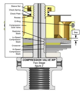
**The Restrictor Valving Stack serves 2 purposes.** First, its diameter can restrict the port size. Second, its thickness can create preload.
