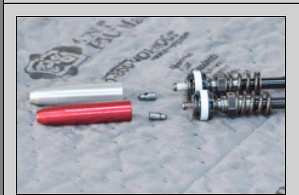
VR3- The Check Valves (the small "bullet" shaped pieces in the middle) will be removed during installation. Shown is the stock direction of the Check Valves.
