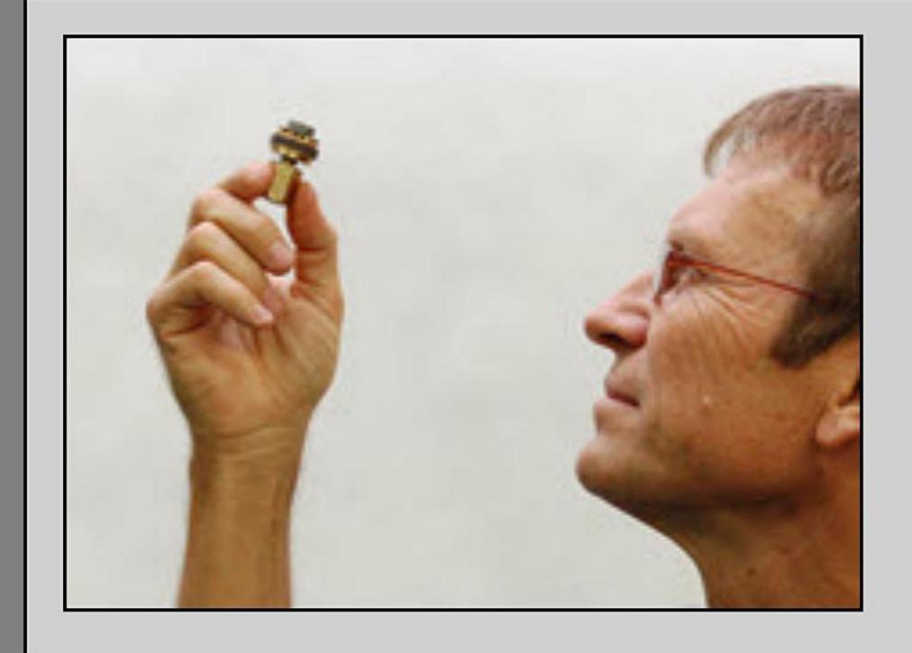
VR19- Check your work. Hold the Valve Stack up to the light and look for proper assembly. If there are any problems, disassemble the stack and look for burrs to surface and/or dirt in the valving. Reassemble and check again.
