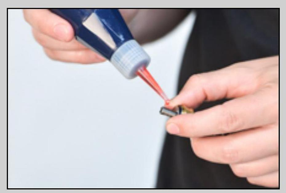
VR13- Apply a small drop of Loctite onto the thread of the rebound valving shaft.
