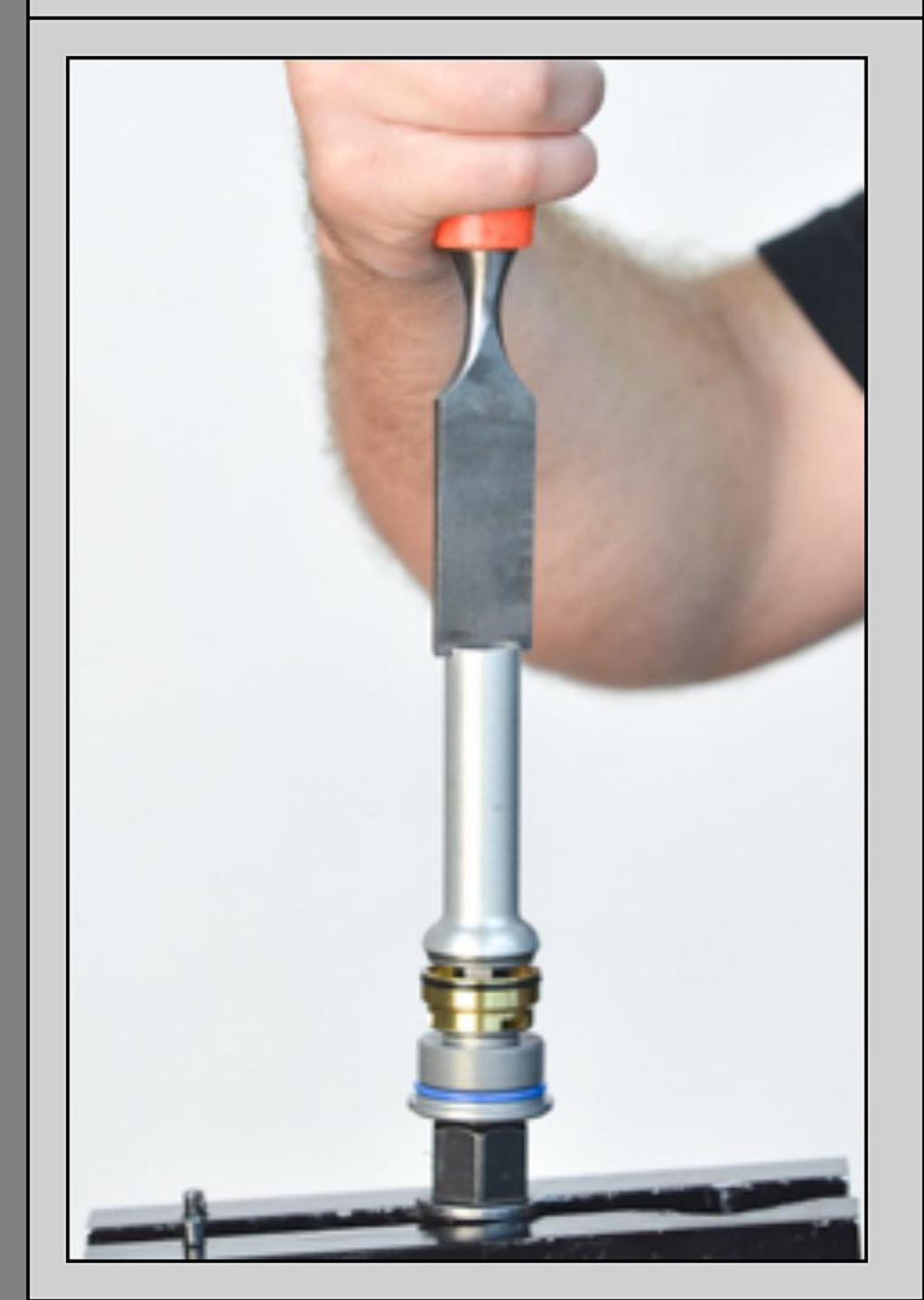
VC15- Using a large screwdriver, tighten the bottom-out cup to 30 in-lbs (2.5 ft-lbs or 0.35 kgf-m).
