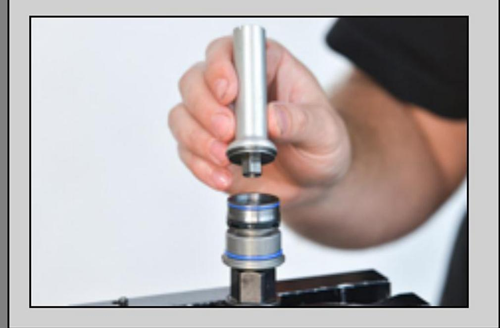
VC3- Remove the bottom-out cup. There are three different styles of bottoming cups plus none.
