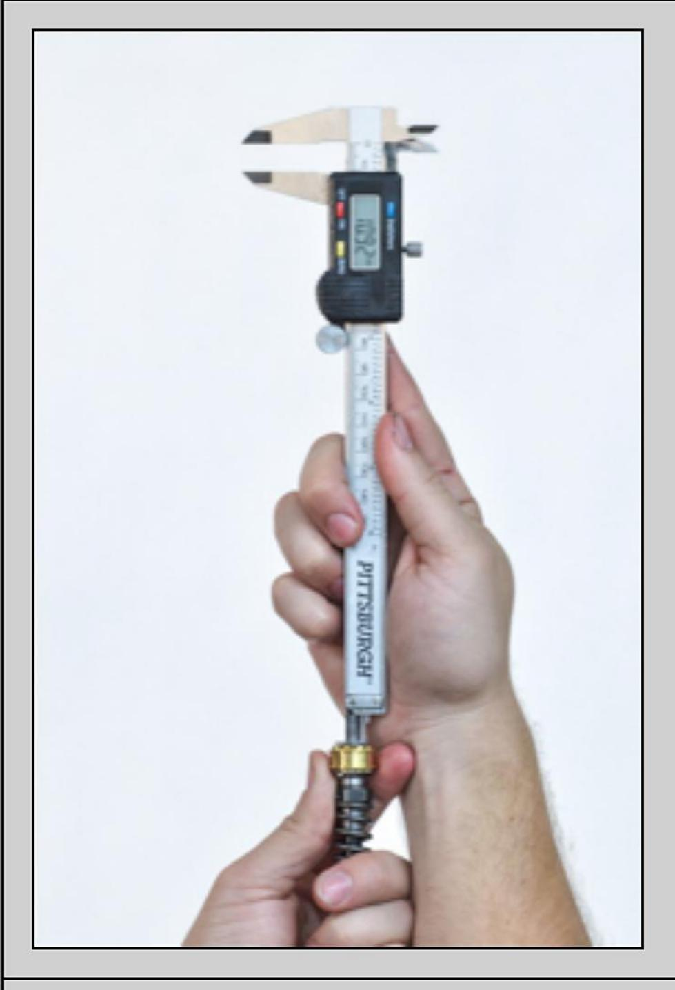
VR12- Measure the post extension beyond the rebound stack. The new measurement must be 10.3 to 10.7mm. CRITICAL!!
