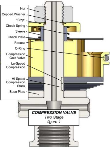
will not tighten down on the valving. This will cause incorrect operation or the nut will come off. This is a critical part of the installation. To get the proper total valve stack thickness you may need to place some of the original shims on the shaft just after the base plate. NOTE: Any shims added must be larger in diameter than the last shim in the stack. **Be sure the nut is fully engaging the threads!**
